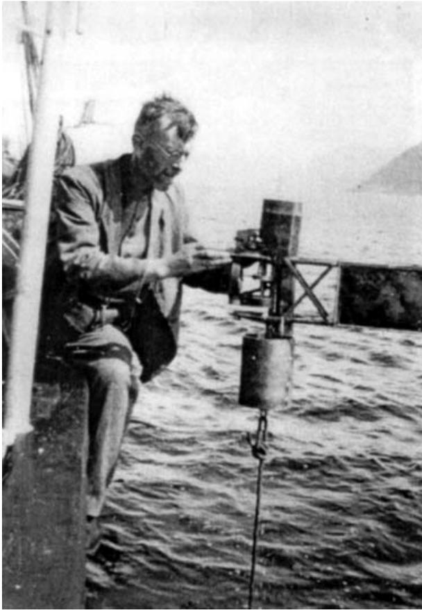
Fig. 1. Ekman operating a repeating current meter. Photograph copyright University of Bergen.
