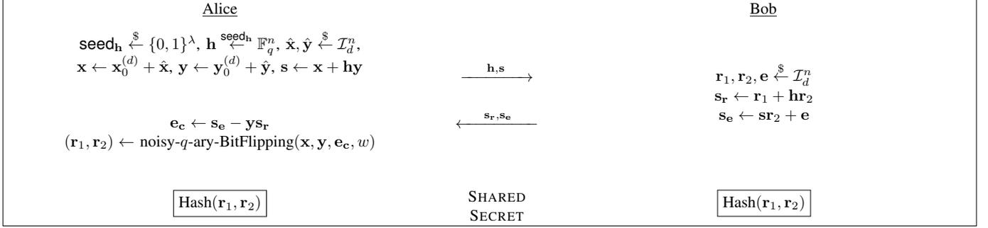
Fig. 1. General description of our Ouroboros-E Key Exchange protocol.  $\mathbf{h}$  and  $\mathbf{s}$  constitute the public key.  $\mathbf{h}$  can be recovered by publishing only the  $\lambda$  bits of the seed (instead of the  $n$  coordinates of  $\mathbf{h}$ ).
