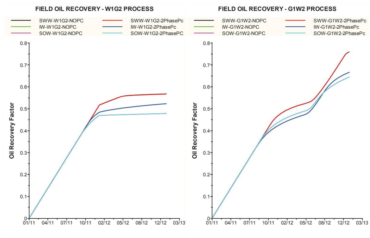
Figure 5. Recovery efficiency for different wettability system and different process, without capillary pressure and using two-phase capillary pressure
