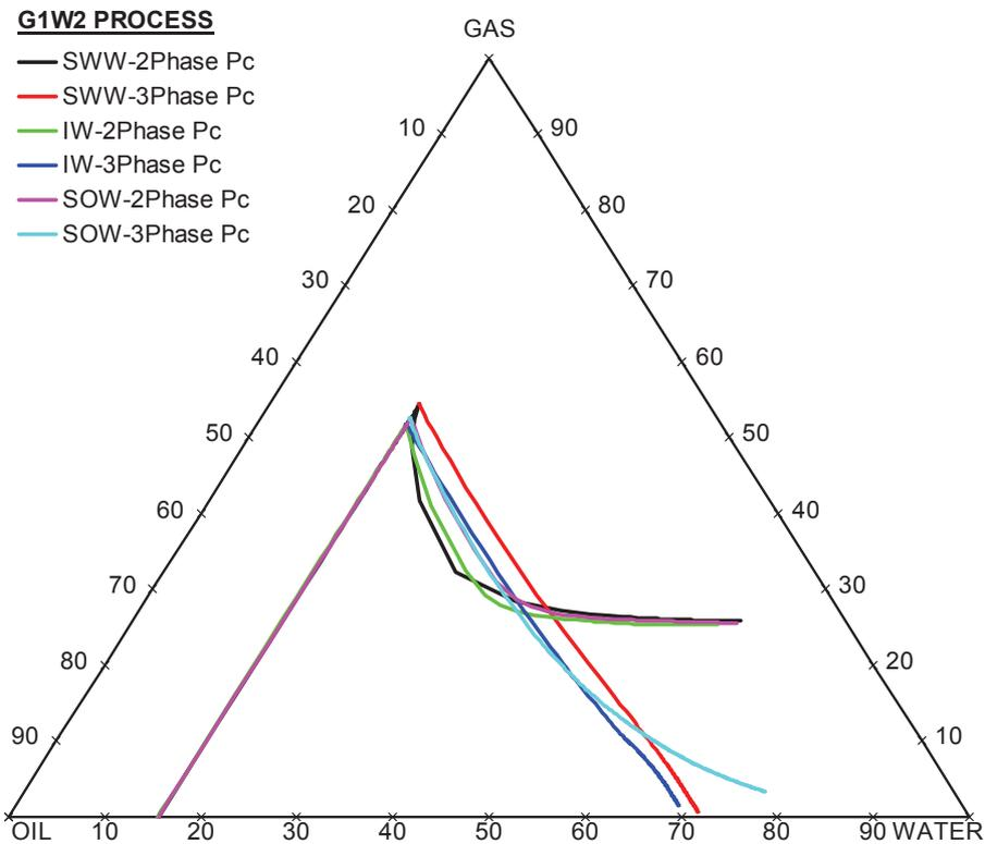
Figure 11. Saturation path at block (2,2,1) for different wettability system, G1W2 process, using two-phase and three-phase capillary pressure
