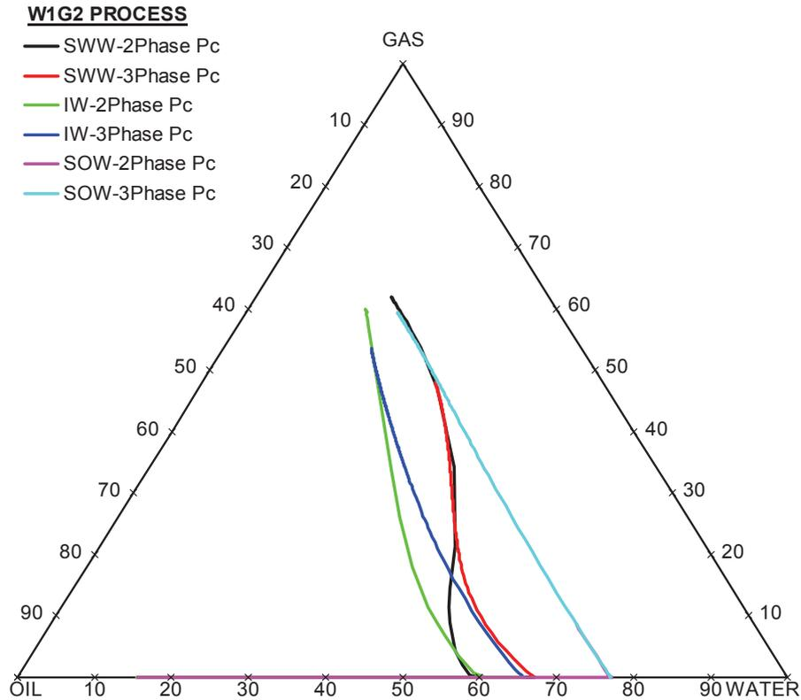
Figure 10. Saturation path at block (2,2,1) for different wettability system, W1G2 process, using two-phase and three-phase capillary pressure
