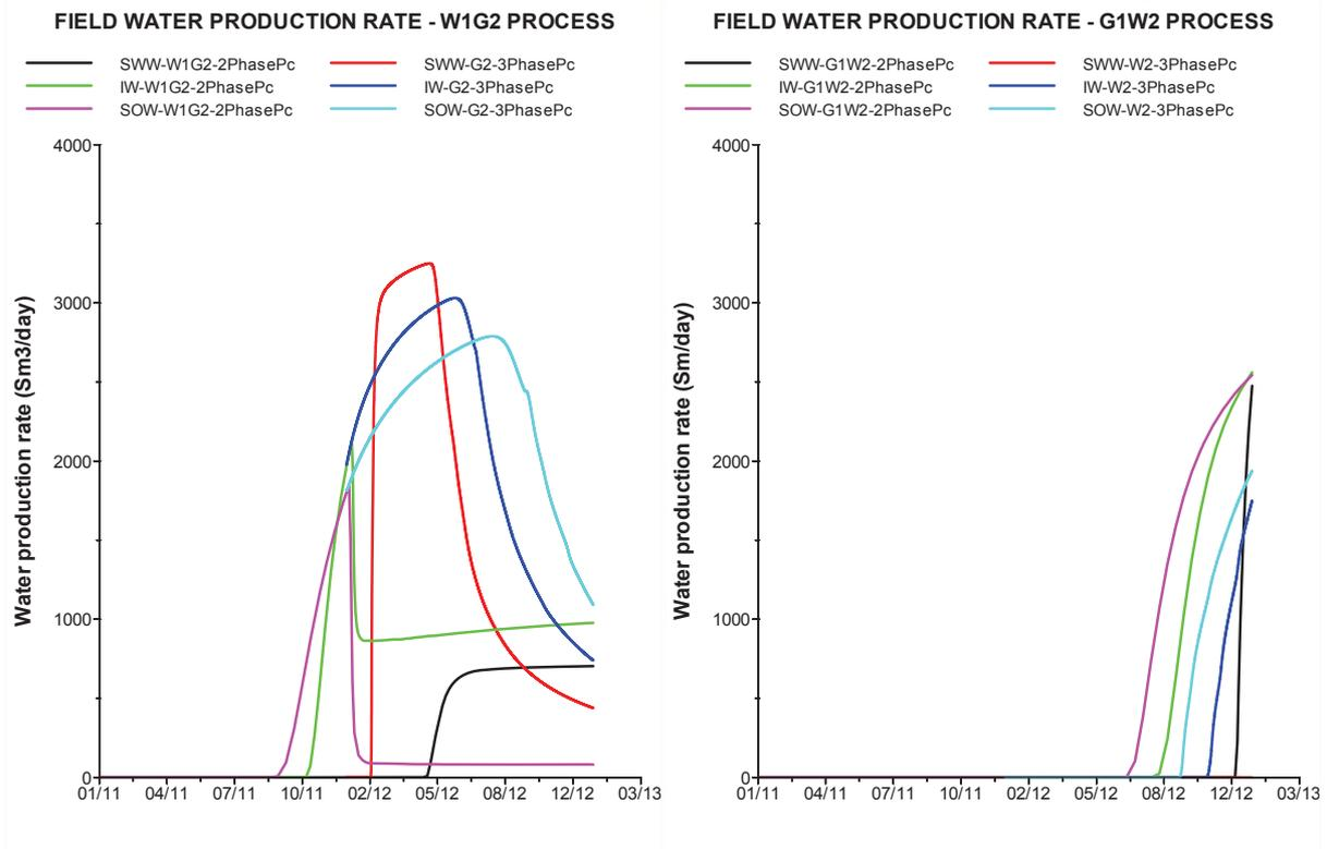
Figure 8. Water production rate profile for different wettability system and different processes, with two-phase and three-phase capillary pressure
