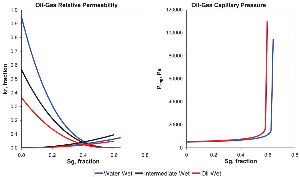
Figure 2. Smoothed two-phase oil-gas relative permeability and capillary pressure from network model for different wettability system
