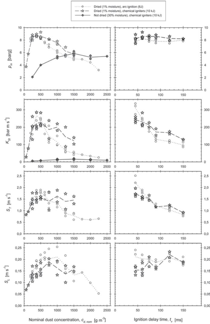
**Figure 3.** Corrected explosion pressures ( $p_m$ ), size corrected rates of pressure rise ( $K_{St}$ ) and estimated laminar and turbulent burning velocities ( $S_T$  and  $S_L$ ) as function of nominal dust concentration (left;  $t_v = 60$  ms) and ignition delay time (right;  $c_{d,nom} = 500$  g m<sup>-3</sup>) for dried copolymer (1% moisture content); some data are also included for wet material (30% moisture content)
