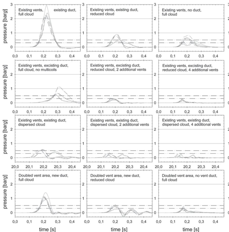
**Figure 7.** Simulated explosion pressures as function of time for various combinations of initial dust clouds, vent areas and vent duct designs; each plot contain results from three different ignition positions, and pressures in two positions,  $M1$  and  $M3$  in Figure 6, are plotted for all simulations. Horizontal lines at 0.3 (and 0.5) barg indicate the design pressure of the dryer (and reinforced dryer)
