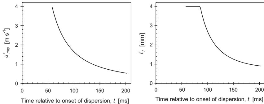
**Figure 2.** The empirical decay laws for the root-mean-square of turbulent velocity fluctuations (left) and turbulent integral length scale (right) in standardized 20-litre explosion vessels
