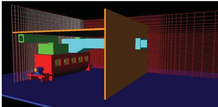
**Figure 5.** Implemented geometry of multicoil drier, illustrating the computational grid; 0.1 m cubical grid cells are used throughout the interior of both the dryer and the vent duct, and the grid cells are stretched outside this region
