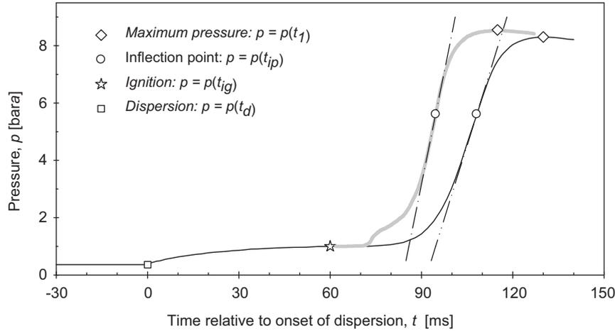
**Figure 1.** Typical pressure-time curves obtained from dust explosion tests in 20-litre explosion vessels; the thin black curve is obtained in a test ignited with a 6 J electric arc, and the thick grey curve illustrates the influence of two 5 kJ chemical igniters on the pressure development
