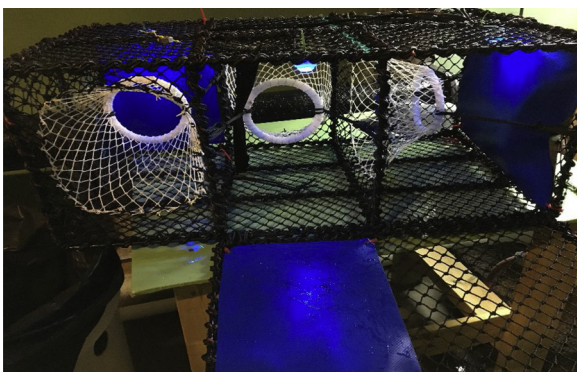
Fig. 1. A modified crab pot used for small-scale testing in tanks.
