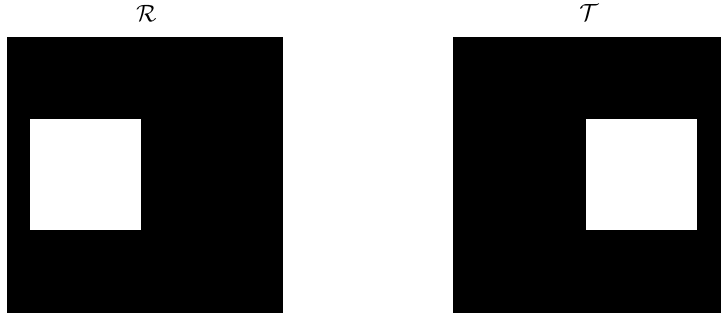
Figure 1.1: Two squares to be registered. Several displacement fields will result in a perfect registration, and hence the problem is clearly ill-posed.
