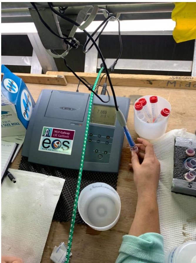
Figure 19: pH were measured using WTW pH/ION meter (Photo taken by Malin Lunde).
