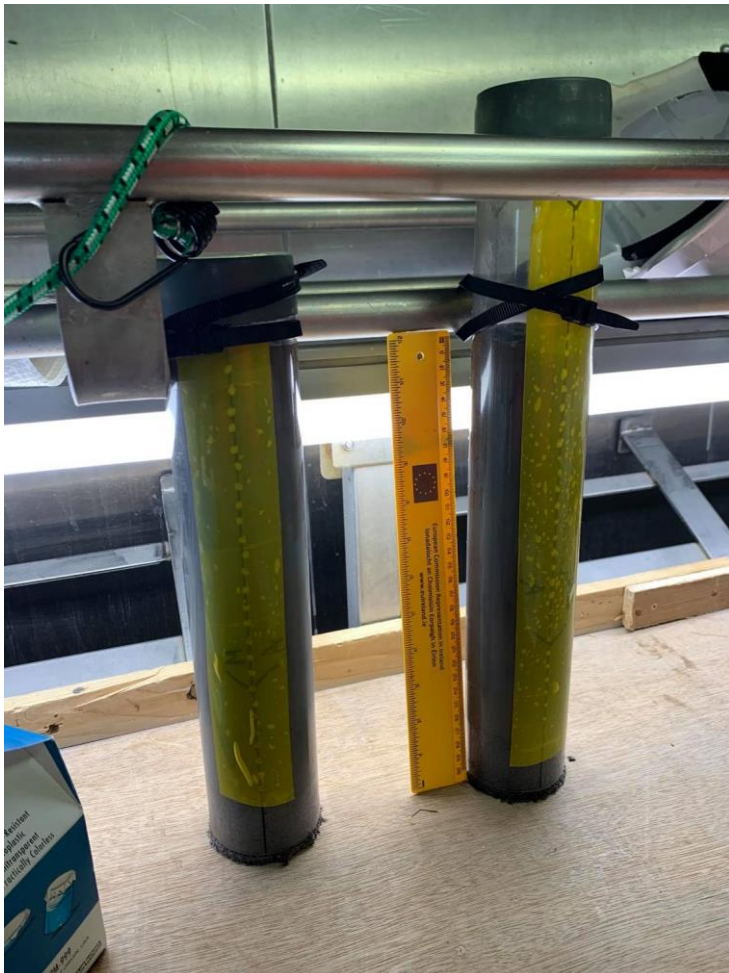
Figure 15: Holes were drilled in the box core and then the holes were taped until further analyzes. The cores were first sampled vertically then on later stations the cores were sampled horizontally.
