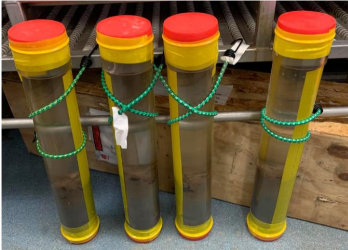
Figure 13: The multicores were stored vertically in the wet lab until analyze. (Photo taken by Malin Lunde)
