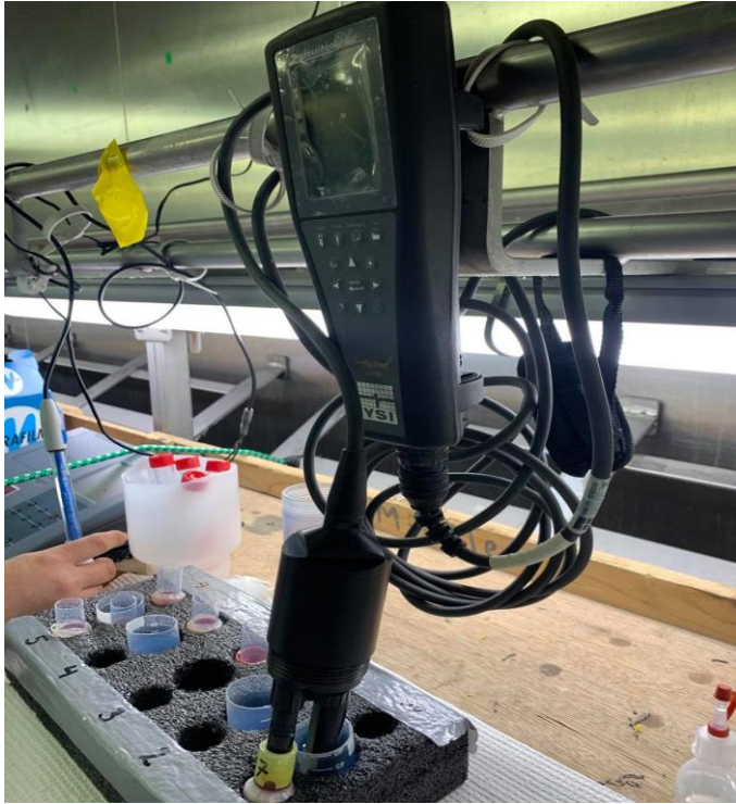
Figure 18: The professional plus multiparameter instrument and the setup of the instrument in the wet lab (Photo taken by Malin Lunde).
