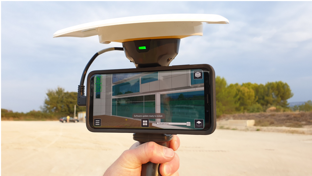
Figure 14: Trimble SiteVision user interface, a handheld Augmented Reality device ( Sitevision.Trimble.com )
