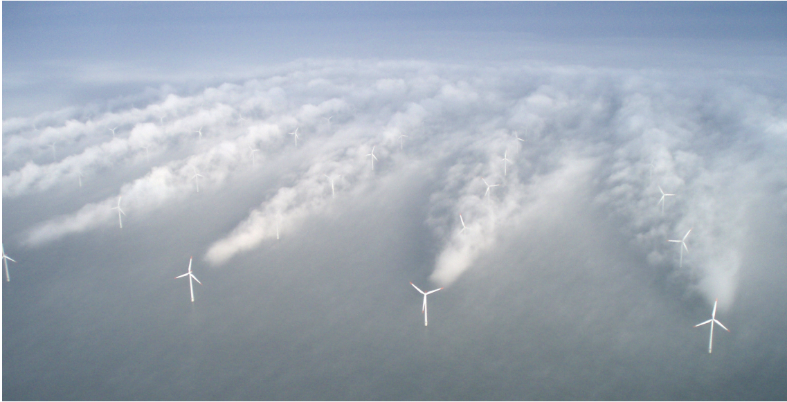
Figure 7: Visualisation of downstream wakes at Horns Rev Offshore Wind Farm in Denmark [27]
