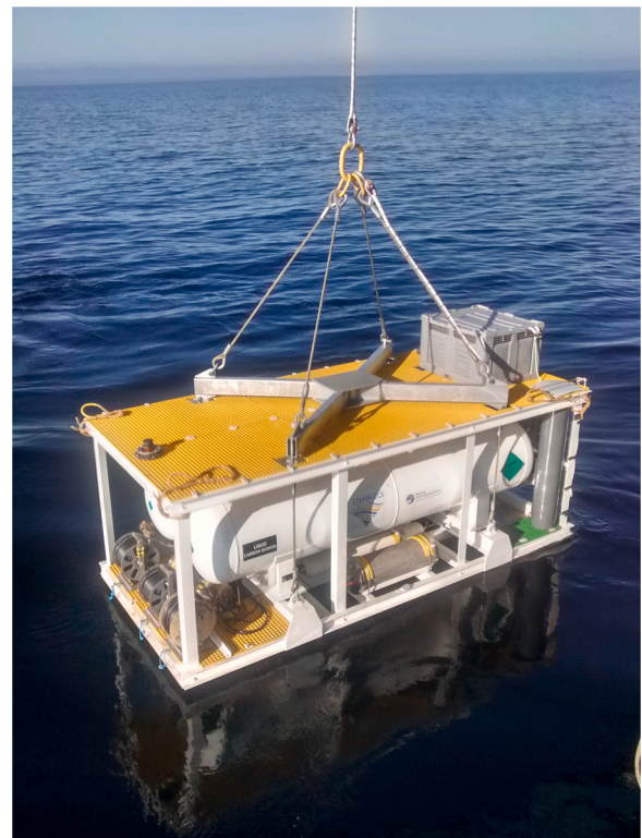
Fig. 6. Deployment of the gas storage and release system.
