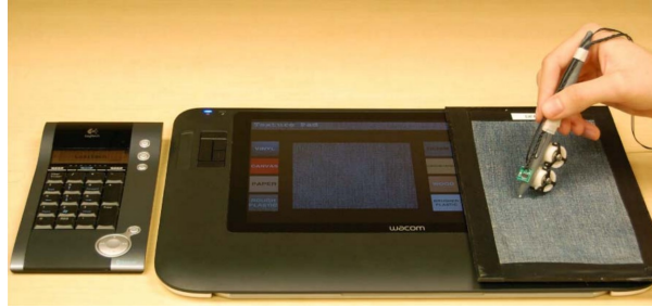
Figure 2.11: Romano and Kuchenbecker [119] simulates textures via vibration on two motors connected to a stylus. The stylus has an accelerometer attached to it such that it can record textures and replicate them using the vibration motors.
