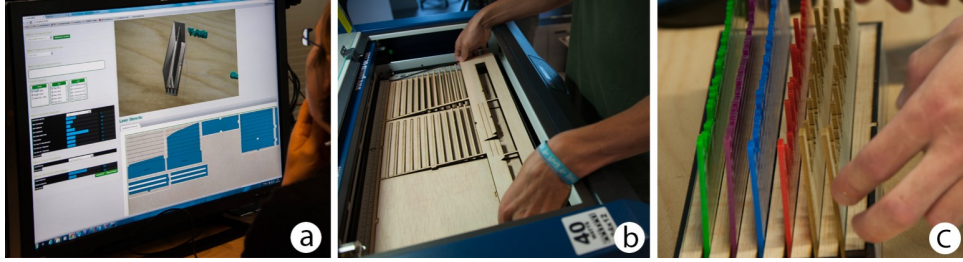
Figure 2.9: MakerVis being used to physicalize a bar chart. The design of the physicalization is chosen in the program, before exporting schematics that can be cut by a laser cutter and finally assembling the layers to form the physicalization. [10]
