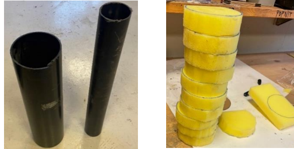
Figure 5.6 – PE pipes before cutting, and foam for fitting inside
