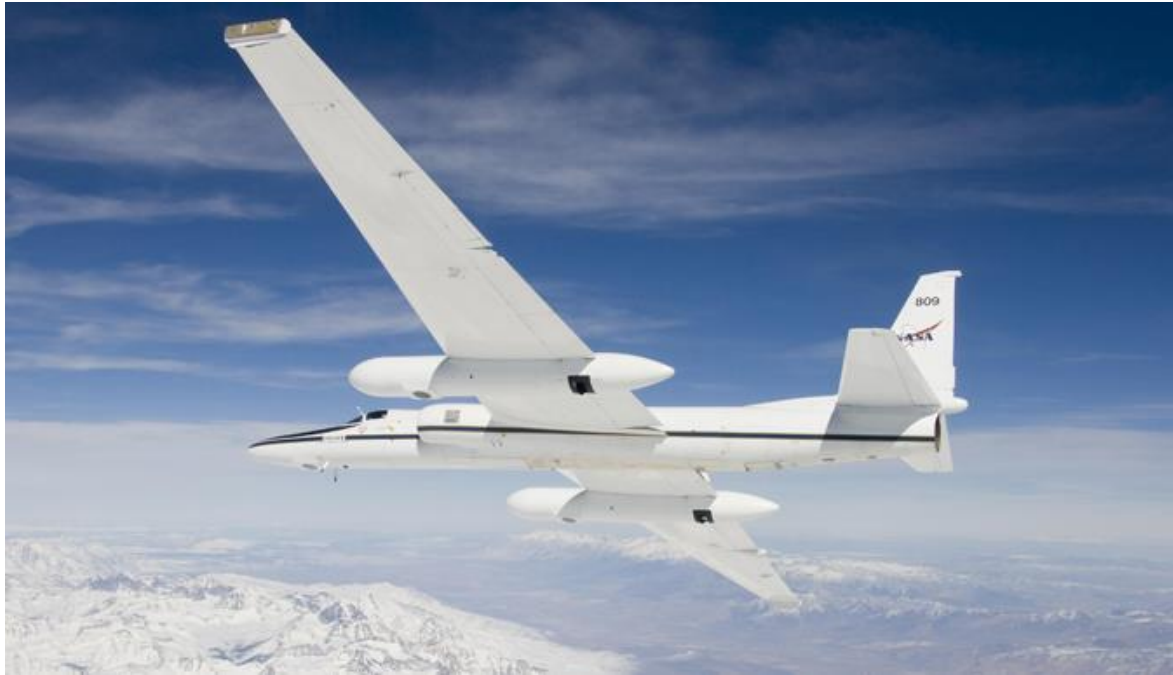
Figure 2-2 A NASA ER-2 in flight. During the 2017 ALOFT campaign the FECS instrument was in the pod beneath the right wing. Picture by NASA/Carla Thomas [15].
