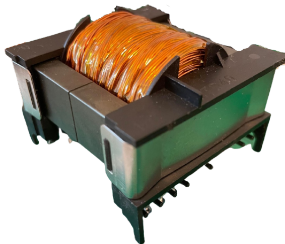
Figure 3.6: Constructed high-frequency transformer
