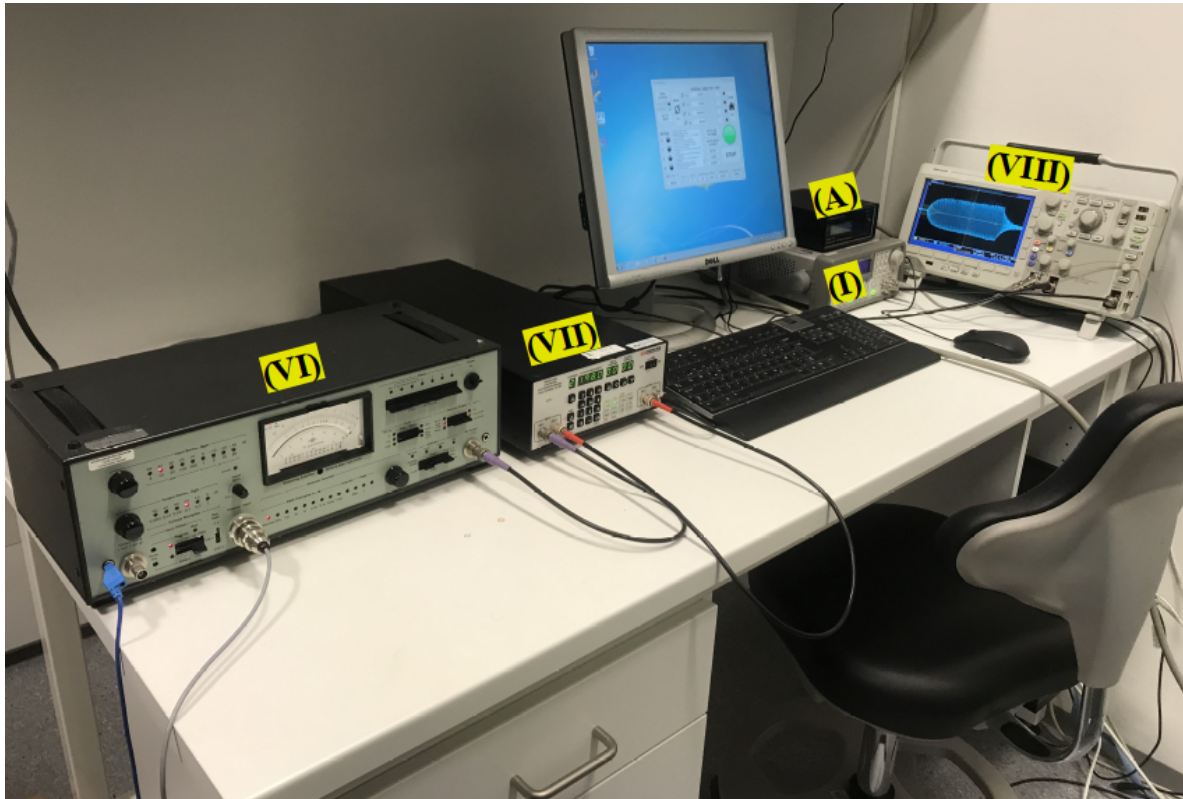
Figure 3.4: A overview of some of the equipment in the acoustical setup, where (A) is the barometer, (I) is the signal generator, (VI) is the amplifier, (VII) is the filter, and (VIII) is the oscilloscope (Table 3.2).
