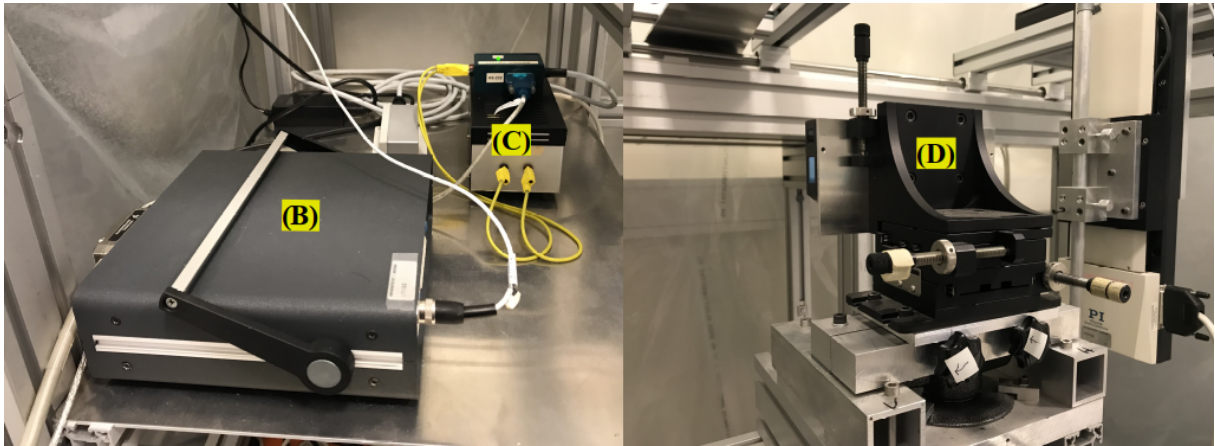
Figure 3.6: A overview of some of the equipment in the acoustical setup, where (B) is the ASLF250 measuring the temperature, (C) the Vaisala measuring temperature and humidity, and (D) is the laser stage.
