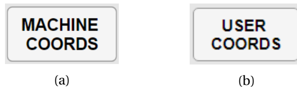
Figure 4.10: (a) indicates that the machine coordinates are active. If pushed, it turns into (b) and indicates that the user coordinates are active.
