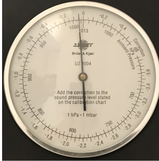
Figure 3.12: Supplied barometer UZ0004 in the pistonphone calibration set [16].
