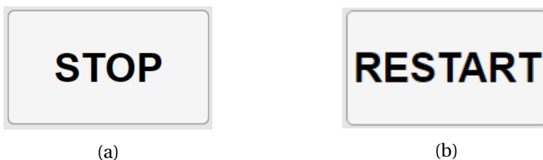
Figure 4.2: (a) Stop button and (b) Restart button. If the stop button is pushed, all motions of the stages stop and halt all actions, and the stop button turns into a restart button. The control over the app is regained when the restart button is pushed.
