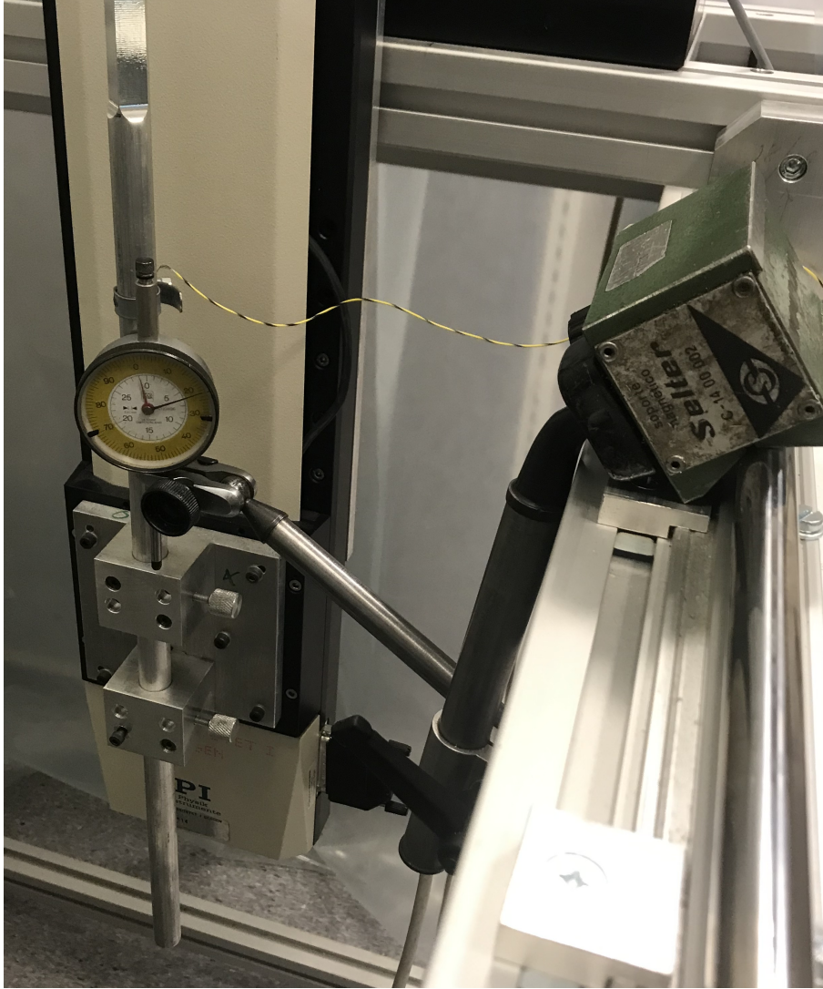
Figure 3.17: Dial gauge lined up parallel to the Y-stage, ready to measure the travel distance of the stage.
