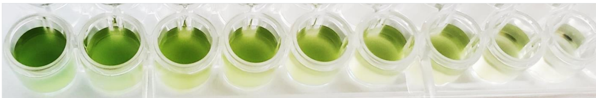
Picture 1 Dilution series conducted to determine the range for accurate OD measurements in the Hides
