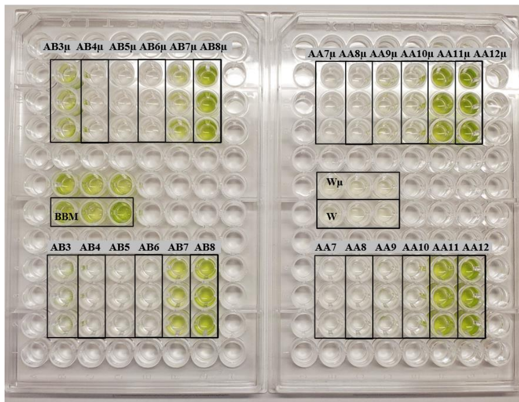
Picture 3 Visual control on the final day of WP3 where the batch 3 WSs were tested with the addition of micronutrients as growth media for C. vulgaris . Abbreviations: AA = Aller Aqua Research, AB= AquaBioTech, \mu = APN, W = water (negative control) , BBM = Bolds basal medium (positive control)
