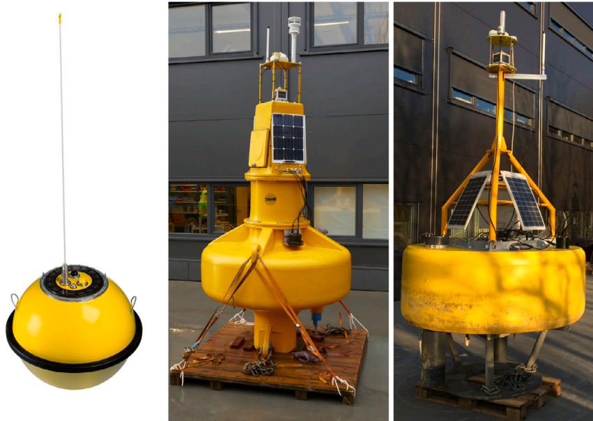
Fig. 2. Left: Waverider Datawell BV (Diameter 70 cm, Datawell BV, 2020) Centre: Tideland SB138P navigation buoy (diameter 175 cm, height 229 cm). Right: EMM2.0 Coastal monitoring buoy (diameter 200 cm, height 328 cm).
