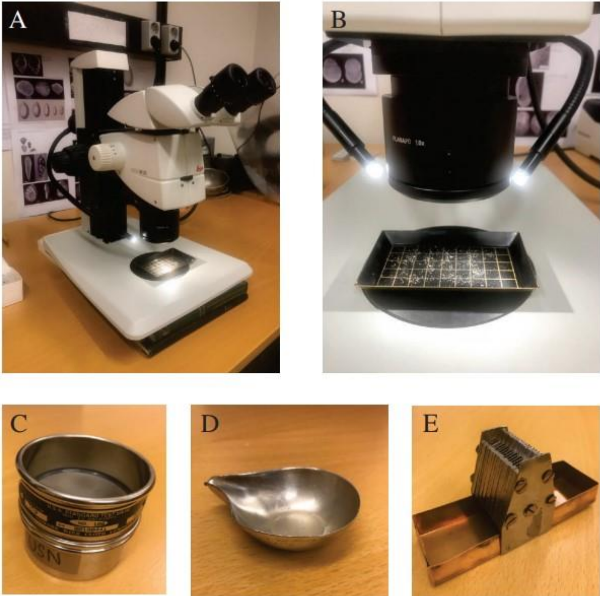
Figure 4.2: Counting equipment used in this project. A) Microscope (type B) B) Counting tray consisting of 45 squares (1x1 cm). C) Sieve to separate the \geq 150 \mu\text{m} fraction. D) Tray used for moving sample between counting tray, sieve and sample container. E) The splitter used to divide the samples prior to counting (Figure 4.1 in Dahm-Johnsen, 2019).
