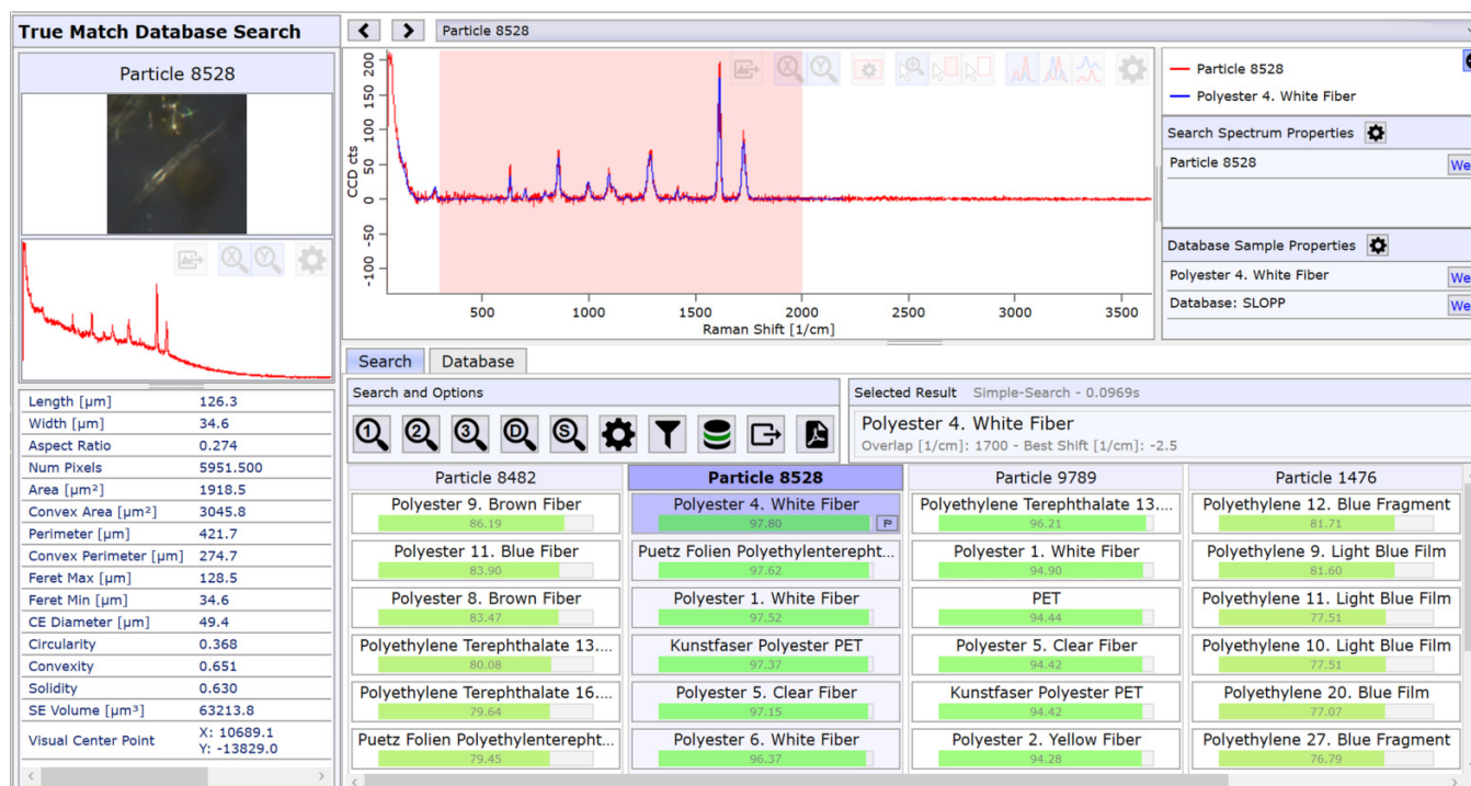
Fig. 2. Example of a microplastic particle identified by Raman spectroscopy using a combination of several spectral databases (Cabernard et al. 2018; Munno et al. 2020; von der Esch et al. 2020a). Left side: Particle image, raw Raman spectra, and particle details derived by image analysis. Right side: Processed spectra (red) and assigned library spectrum (blue) for the selected particle and reference spectra (highlighted in violet) combined with material name and further information.
