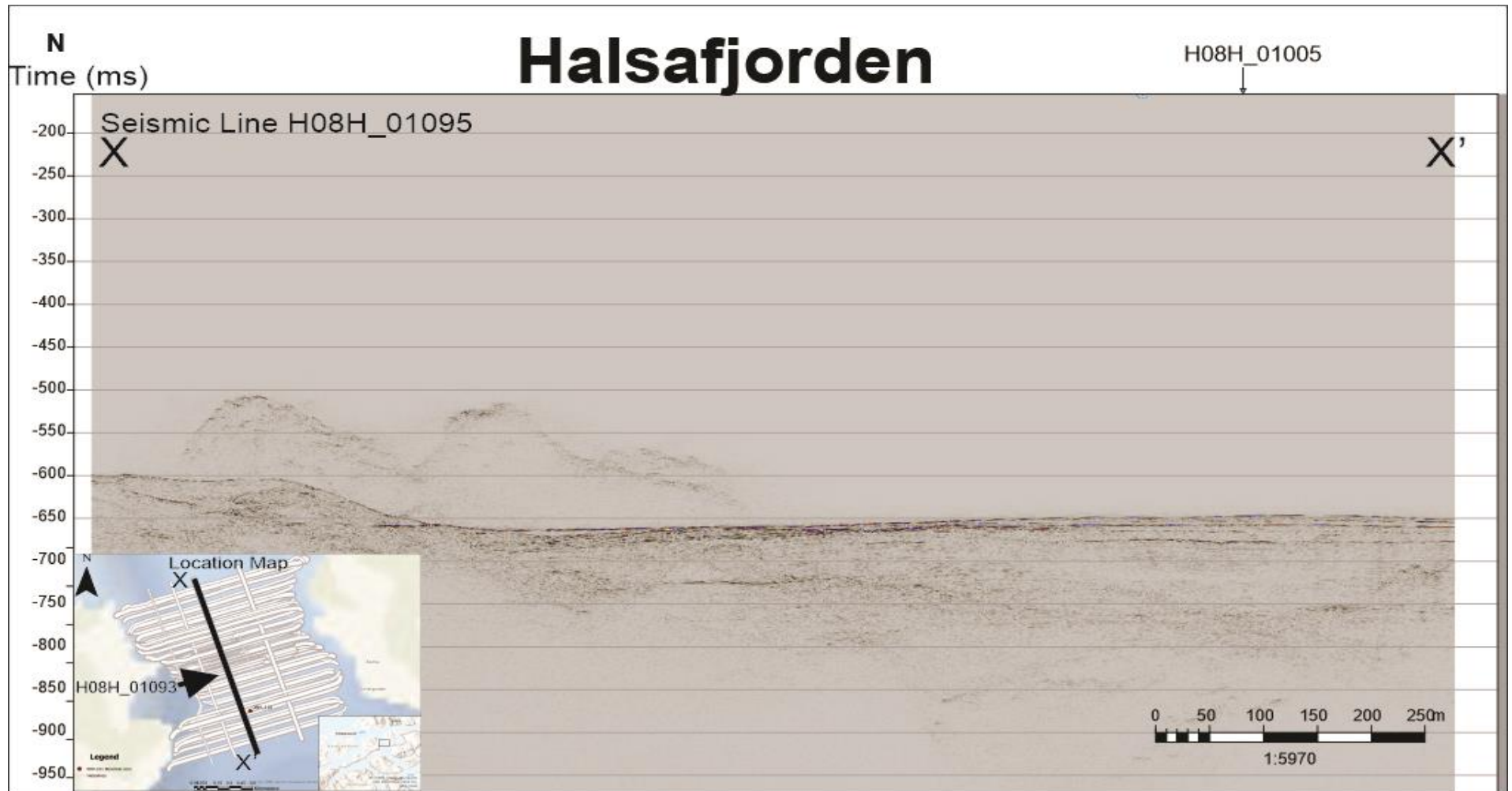
Fig. 22. Uninterpreted seismic profile of Line H08H_01095 showing the subsurface geology and possibly a glacial till. It also shows the line H08H_01005
