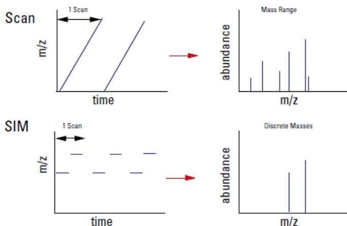
Figure 2.6.5: Illustration showing Scan and SIM data acquisition.
