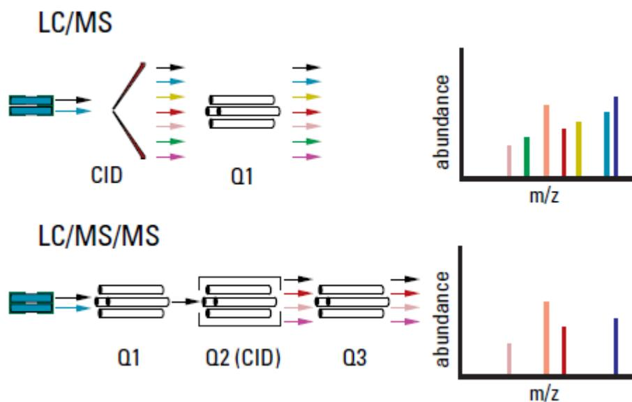
**Figure 2.6.6:** CID with single quadrupole and triple quadrupole mass spectrometers (Packard 1998)
