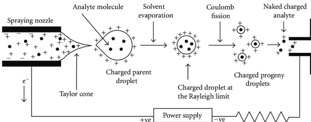
**Figure 2.6.1:** Electro spray ionization (ESI) (“Figure 6: Schematic Representation of the Electro spray Ionization Process.” 2022)
