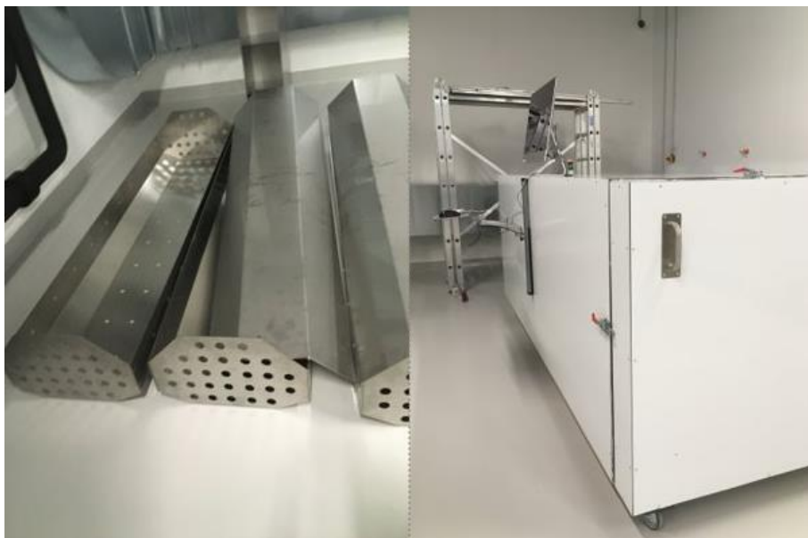
Figure 4: The "Dutch prove" dewar interior; the cooldown box.
