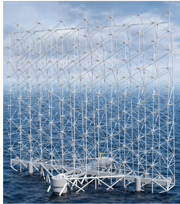
Figure 1.3: Windcatching systems' multirotor design [16].
