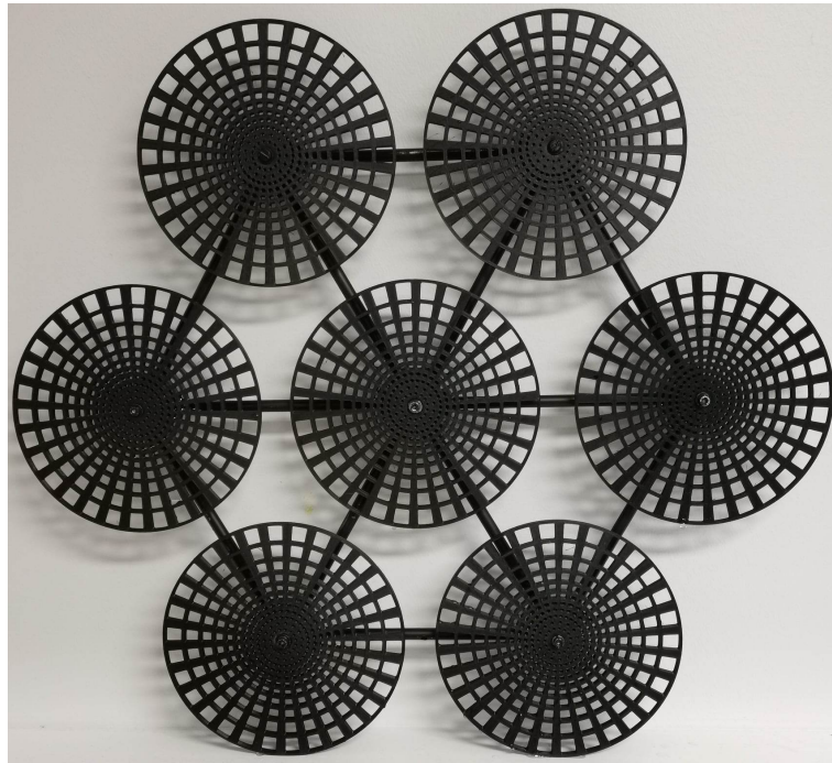
Figure 3.2: Porous discs used in the measurement campaign, arranged in an MR7 setup.
