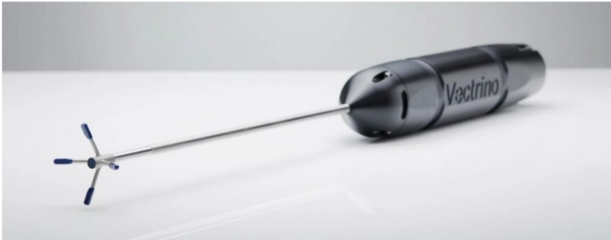
Figure 3.11: The Vectrino+ velocimeter from Nortek [51].
