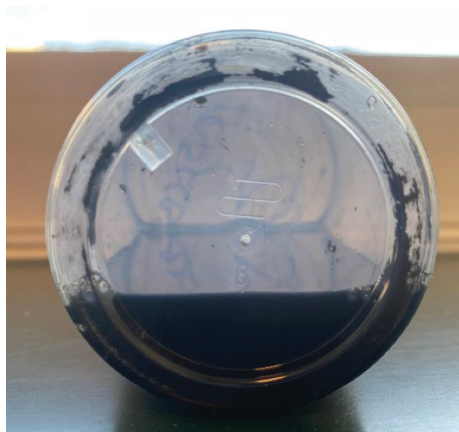
(c) Sedimentation on the container bottom after seven days (a sample was collected after the experiments)
