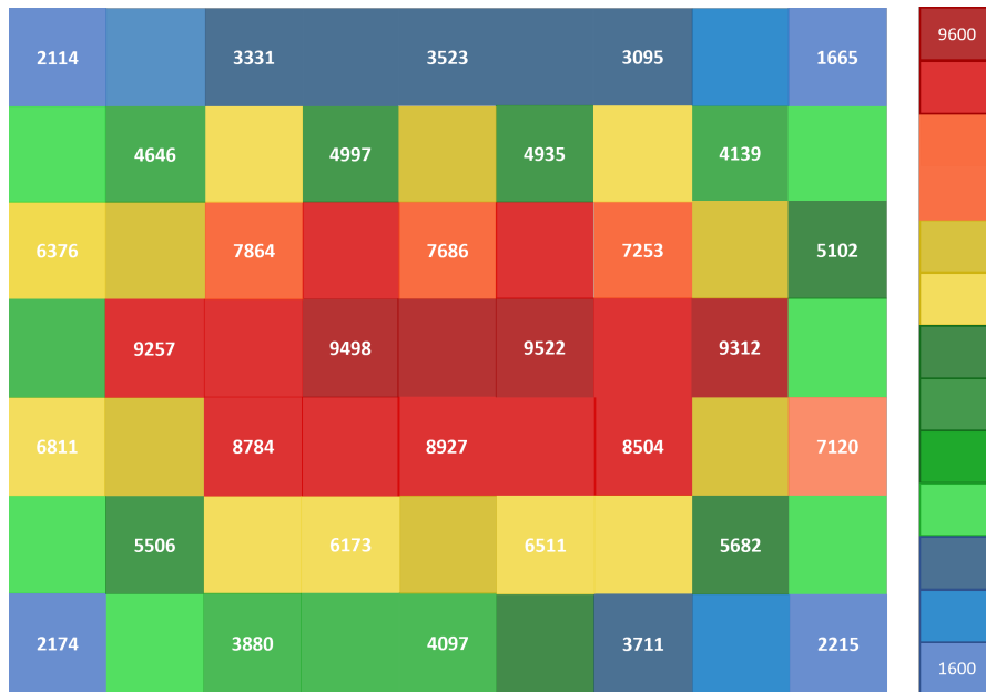
Figure H.2: Intensity distribution in [W/m^2] at a distance of 8 cm from the light source.
