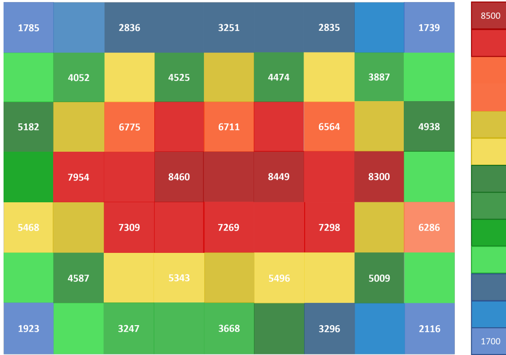
Figure 3.4: Intensity distribution in [\text{W}/\text{m}^2] at a distance of 10 cm from the light source.
