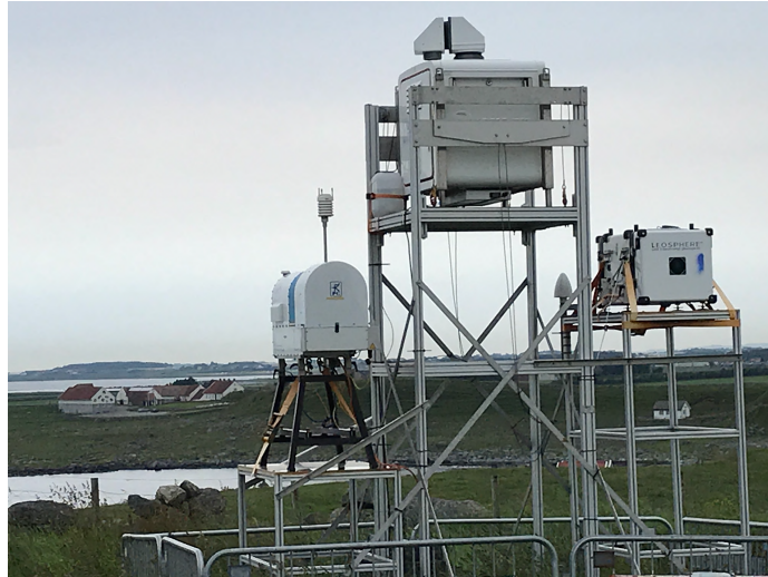
Figure 3.2: WindCube 100S (LidarN) in the center installed 3 m above the ground to compensate for lower terrain at the position WindCubeV1 to the right and Radiometer Physics HATPRO RG4 to the left. Instruments are installed on the Bosch Rexroth aluminum strut profiles. View towards the North direction. Source: (Cheynet et al., 2021)
