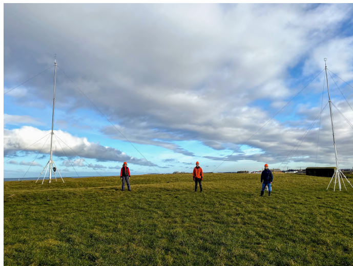
Figure 3.3: Two telescopic masts equipped with 3D sonic anemometers on their top at a height of 11 m above the ground with a separation distance of 20 m between them and approximately with 100 m distance from the LidarN. Source: (Cheynet et al., 2021)
