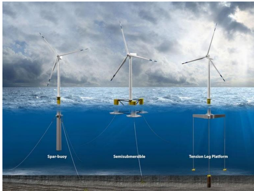
Figure 2.8: Offshore WT floating structures (IRENA, 2016).
