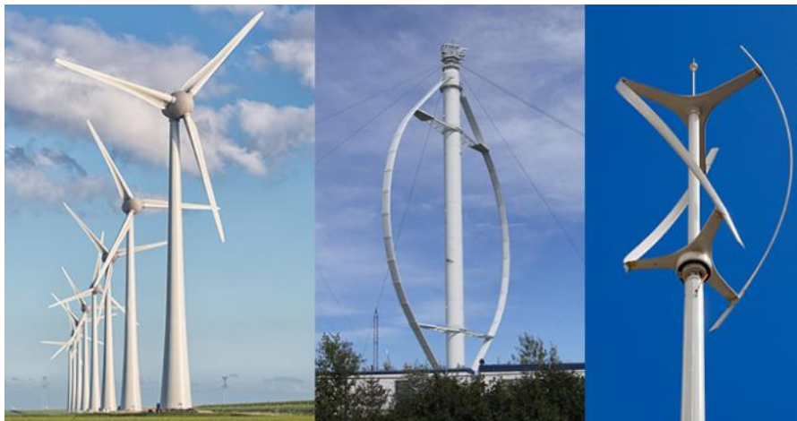
Figure 2.2: Horizontal axis wind turbine (left) and vertical axis wind turbine (middle and right) (Marietta, 2023)
