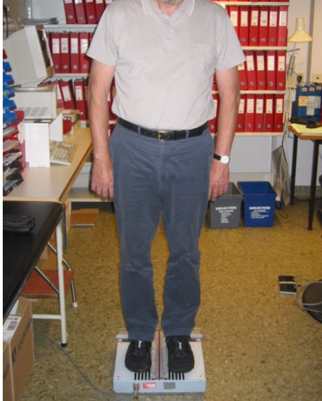
Figure 16.5. The static posturography. A force platform with three pressure transducers is connected to a computer. The path length based on the COP values were used for analysis.
