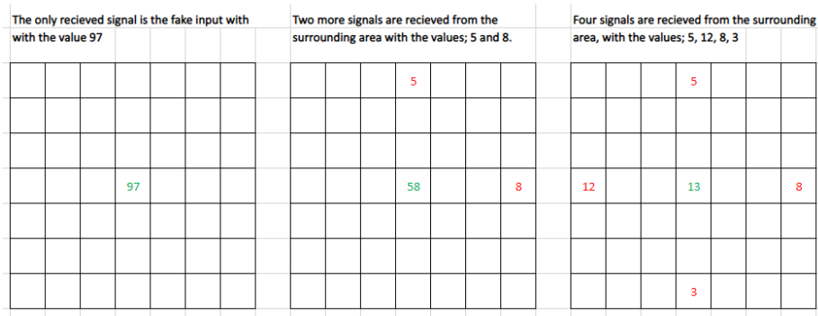
Figure 39: Concept illustration of the handling of false positive signal value
