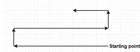
Figure 43: Illustrating grid flight pattern
