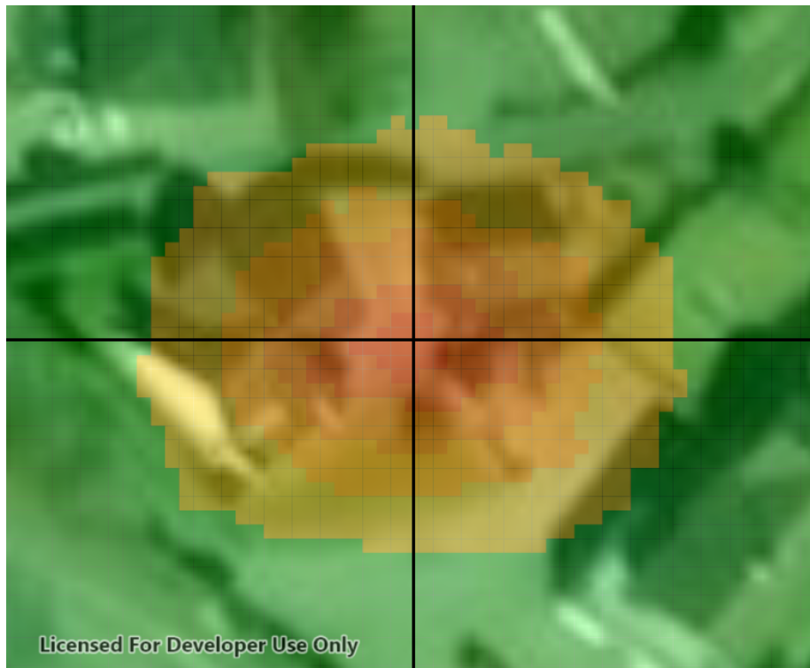
Figure 30: Capture of the output with a 90 degree orientation of the avalanche device and a speed of 5m/s
