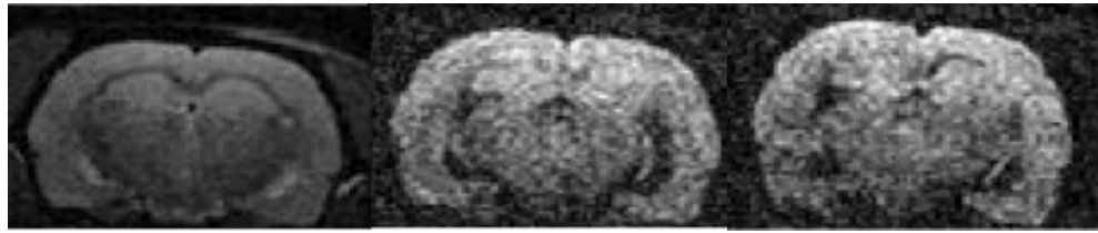
Figure 4-7 Second isotropic sequence V_s = 0,64 \text{ mm}^3 , V_x, V_y = 0,4 \text{ mm} , ST = 0.4 \text{ mm} , N_{Pe} = 64 , N_{Fe} = 64 , TR = 4000 \text{ ms} , TE = 30 \text{ ms} , NEX = 10 , Shots = 4 , FOV_x = 12,8 , FOV_y = 12,8 , Time = 128 \text{ min} , Number \text{ of slices} = 28 , Area \text{ covered in Z dimension} = 11,2 \text{ mm} .
