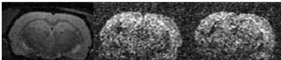
Figure 4-6 Sequence with ST = 2 \times V_x, V_y V_s = 0,16 \text{ mm}^3 , V_x, V_y = 0,2 \text{ mm} , ST = 0.4 \text{ mm} , N_{Pe} = 64 , N_{Fe} = 64 , TR = 4000 \text{ ms} , TE = 30 \text{ ms} , NEX = 10 , Shots = 4 , FOV_x = 12,8 FOV_y = 12,8 , Time = 128 \text{ min} , Number \text{ of slices} = 28 , Area \text{ covered in Z dimension} = 11,2 \text{ mm} .
