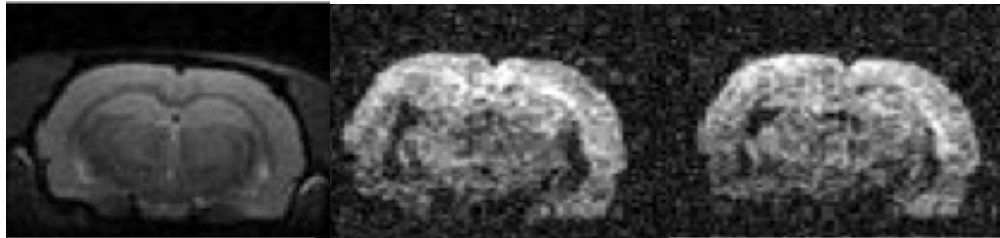
Figure 4-8 Second sequence with ST = 2 \times V_x, V_y V_s = 0,31 \text{ mm}^3 , V_x, V_y = 0,25 \text{ mm} , ST = 0.5 \text{ mm} , N_{Pe} = 64 , N_{Fe} = 96 , TR = 4000 \text{ ms} , TE = 30 \text{ ms} , NEX = 10 , Shots = 4 , FOV_x = 16 , FOV_y = 24 , Time = 128 \text{ min} , Number \text{ of slices} = 28 , Area \text{ covered in Z dimension} = 11,2 \text{ mm}
