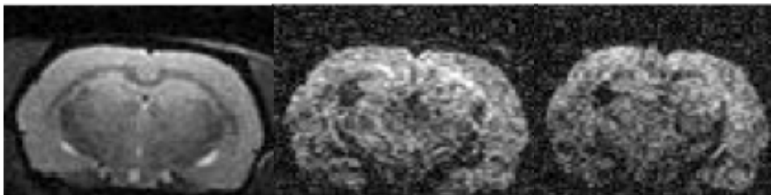
Figure 4-2 Sequence with extended number of slices V_s = 0,24 \text{ mm}^3 , V_x, V_y = 0,22 \text{ mm} , ST = 0.5 \text{ mm} , N_{Pe} = 64 , N_{Fe} = 96 , TR = 4000 \text{ ms} , TE = 30 \text{ ms} , NEX = 10 , Shots = 4 , FOV_x = 14 , FOV_y = 21 , Time = 128 \text{ min} , Number \text{ of slices} = 28 , Area \text{ covered in Z dimension} = 14\text{mm} .
