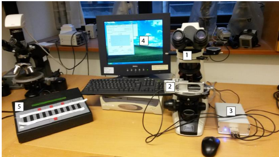
Fig. 3.8: Shows the point counting equipment in the Microscopy Lab at the University of Bergen. 1) Nikon EclipseE200POL, polarizing microscope 2) MicroStepper stage, Mk1.5 "wire-connected" 3) MicroStepper stage controller box 4) PETROG Lite software 5)PRIOR MODEL G point counter
