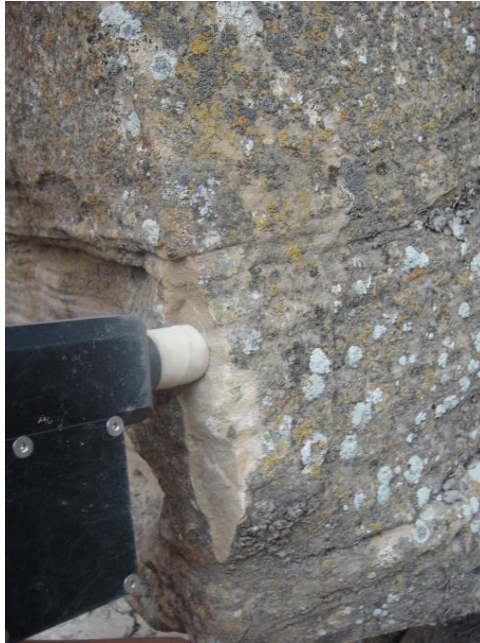
Fig. 3.2: Permeability measurement on a clean and planar surface. This measurement is from a LSF sandstone in Spring Canyon Mb. of the Blackhawk Fm. located in Gentile Wash.
