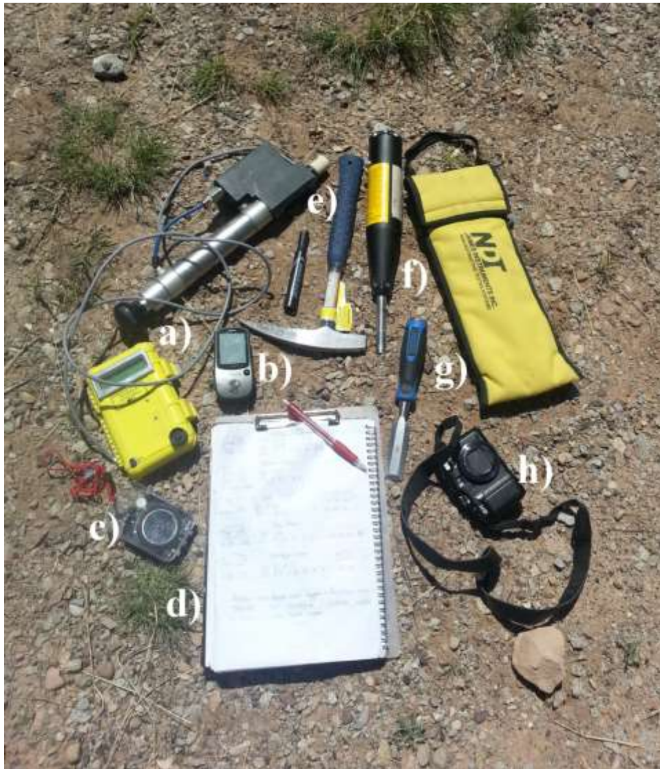
Figure 1.9: The equipment used for performing measurements with Tiny-perm II and Schmidt Hammer: a) Tiny-perm II, b) GPS recorder, c) compass, d) notepad, e) geology hammer, f) Schmidt Hammer, g) chisel and h) camera.
