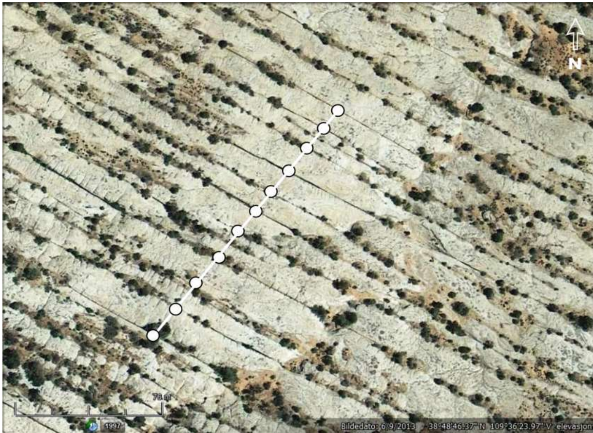
Figure 1.11: Example of a scanline and the fractures recorded (marked by white dots) in the Moab Member, based on aerial photos from Google Earth.
