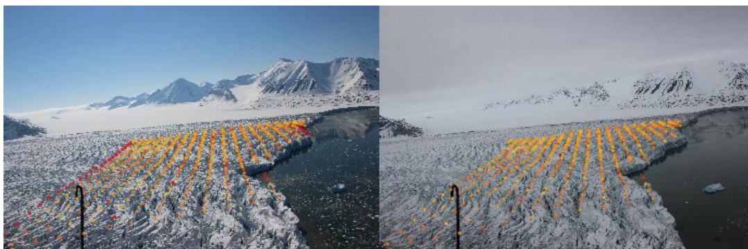
Figure 3.11 The template match process between the images from Figure 3.9 (June 4 th and 5 th ), here with a 75x75 m grid of points. The colour of each point represents the quality of the match, where yellow is good and red bad.
