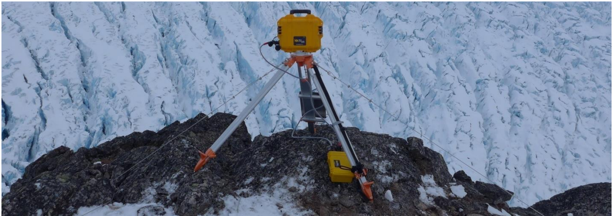
Figure 2.2 Time lapse camera set up on the nunatak Steindolpen looking down at Kronebreen
