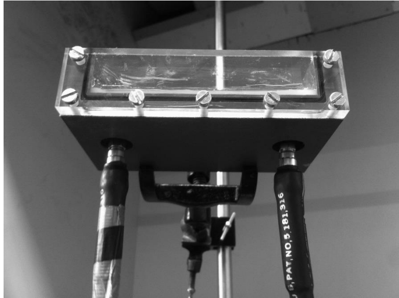
Figure 4.4 Photograph of the vertical coaxial connection on sensor B.
