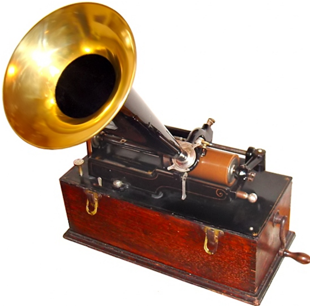
Figure 2 – Edison phonograph circa 1899 using wax cylinder. Licensed under Public Domain via Wikimedia Commons.
