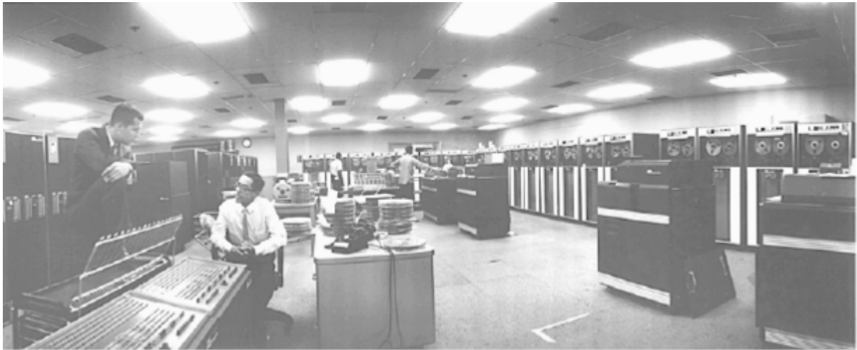
Figure 7 - An IBM 7090 electronic computer taking up the whole room. Licensed under Public Domain via Wikimedia Commons
