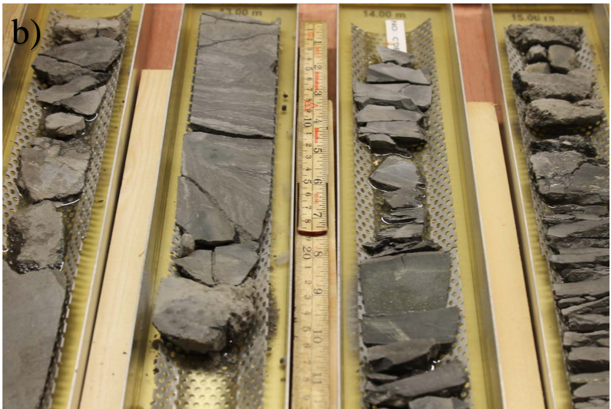
Figure 19: a) The interval between 19.38 and 19.50 meter in core 7831/2-U-1, comprising mudstone with calcite veins and phosphate nodule horizon, possibly formed as tunnel infillings. b) The uppermost 30 cm of the interval between 15 and 12 meters in core 7831/2-U-1, showing sandstone, siltstone, pyritic mudstone and highly fractured shale.
