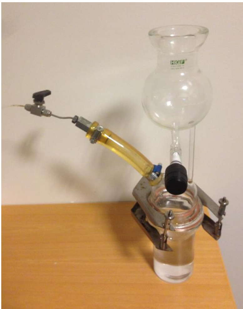
Figure 25: Set-up for vacuuming water with transition-valve to the experimental pump.
