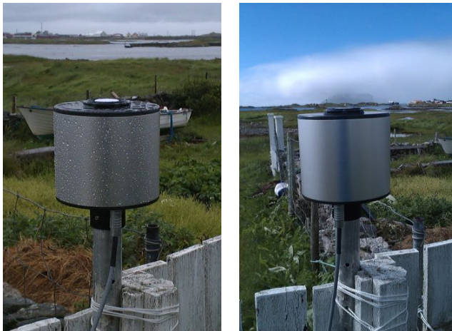
Figure 2.1: The NILU-UV instruments during a field trip at Røst, northern Norway in July, 2012. The instrument is robust and can be seen being used in both wet and dry weather conditions.
