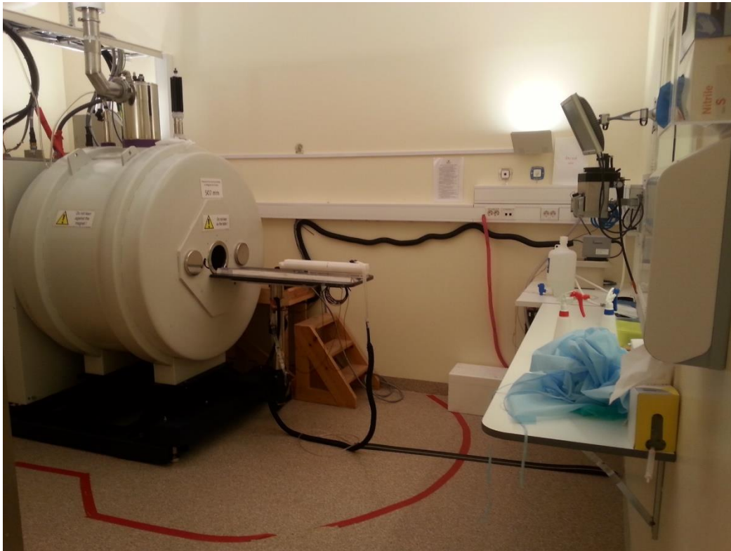
Figure 3.3: The Bruker Pharmascan® 7T small-animal MRI used in this study. Connectors for animal bed water-heating and anesthesia (sevoflurane) visible. Animal bed and coils not mounted in picture.
