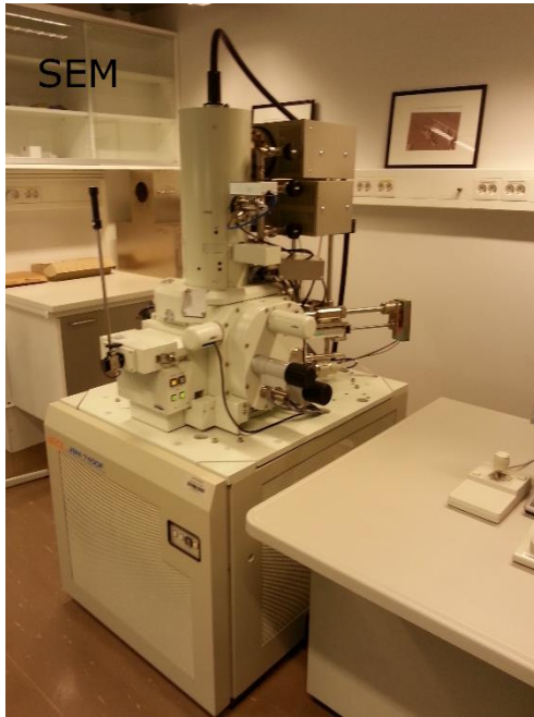
Figure 3.2: The electron microscopes used for this study. SEM: The Jeol JSM-7400F scanning electron microscope. TEM: The Jeol JEM-1230 transmission electron microscope. Both microscopes situated at the Molecular Imaging Centre core facility (University of Bergen).
