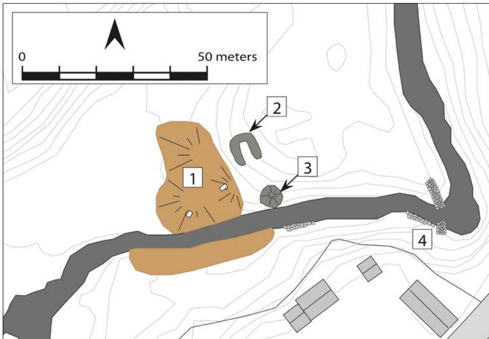
**Figure 6.** The iron mill at Hanakne, Grua in Oppland. 1: Slag heaps. 2: House site, possibly a storage area for ore and charcoal. 3: Furnace. 4: Ruins of a mill and a dam, possibly from the 18th century.
