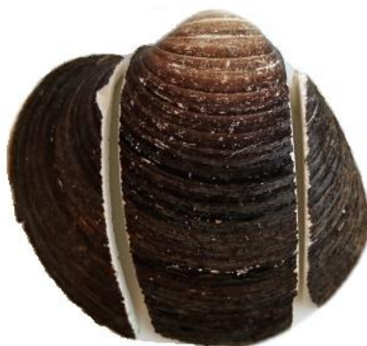
Figure 14: Sectioned left shell valve. The middle part is chosen for further processing.
