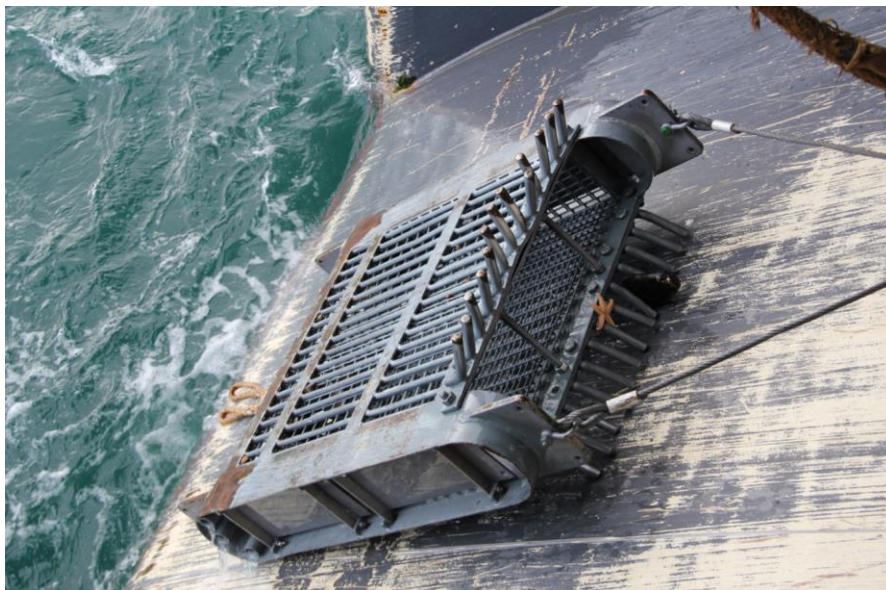
Figure 12: Big Arctica shell dredge used to collect shell material from the sea floor. Photo: taken by me during the Ice2ice cruise expedition GS16-204 in August 2016.
