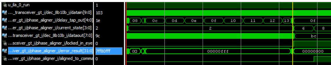
Figure 5.16: Internal signals during the automatic phase and word alignment with a 2.0m long cable. Measurement is done after clock phase shift. Obtained by ILA.
