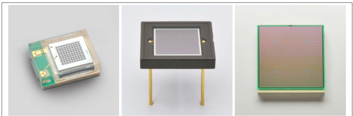
Figure 3.2: Photographs of typical SiPMs. Hamamatsu Photonics K.K. 2017 [27, 28, 29].
