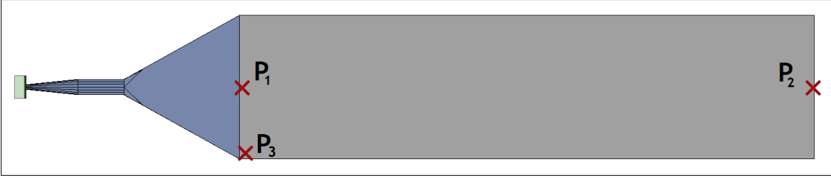
Figure 2.7: Positions P_1 ( y = -49.9 cm, x = 0 cm), P_2 ( y = 49.9 cm, x = 0 cm), and P_3 ( y = -48 cm, x = -10.5 cm), denoting the positions of impacting muons used in the investigation of A_{LG}(t) .
