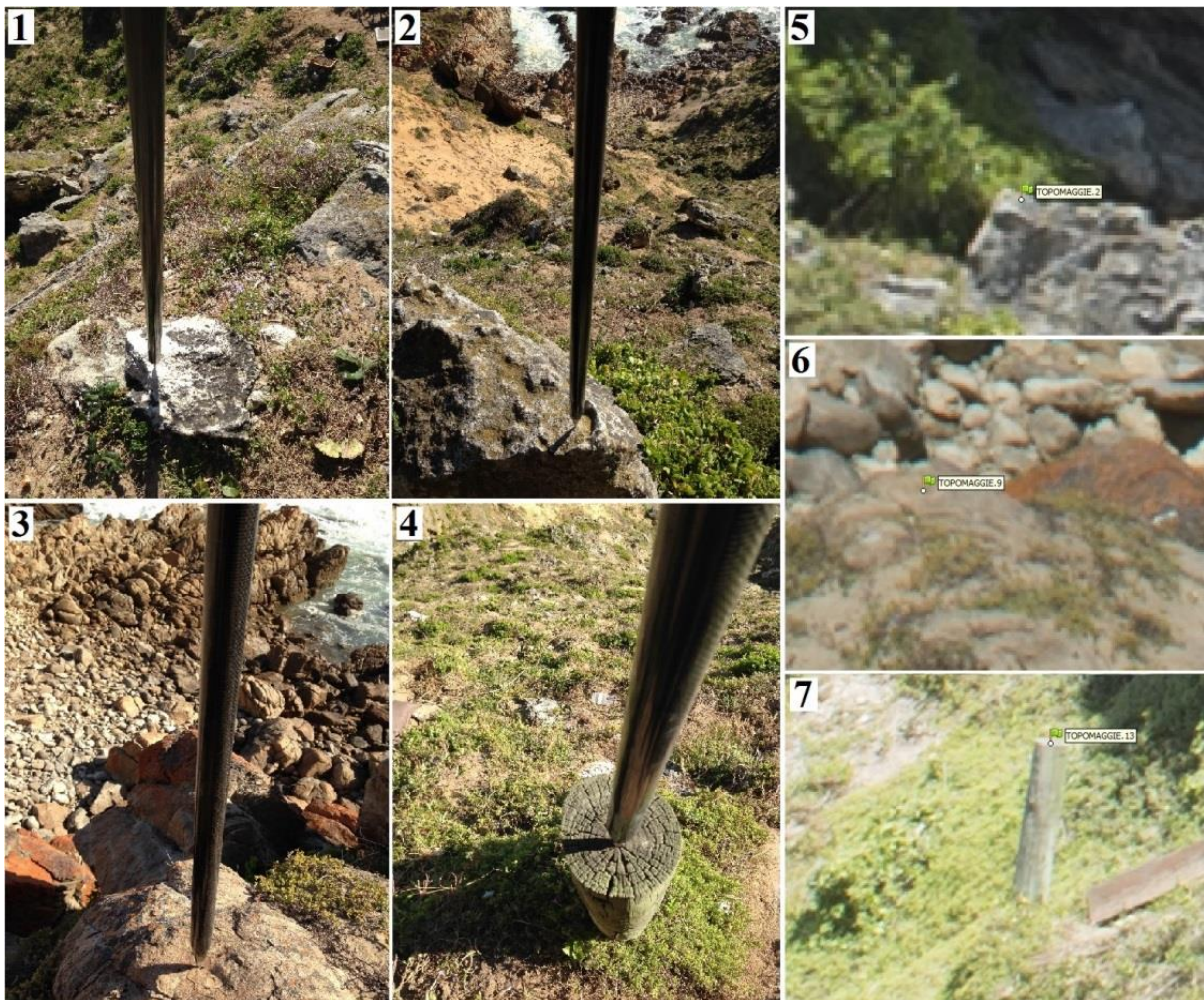
Figure 15. Images were captured using a smartphone to help document the position of the reference points recorded across landscape surrounding BBC (1, 2, 3, 4). These images were used as a reference to help identify and mark the reference positions within photogrammetric image set that covered the BBC exterior landscape (5, 6, 7). In this example 2, 3, and 4 represent 5, 6 and 7 respectively. Several of the other reference positions, including 1, proved impossible to locate in the photogrammetric image set.
