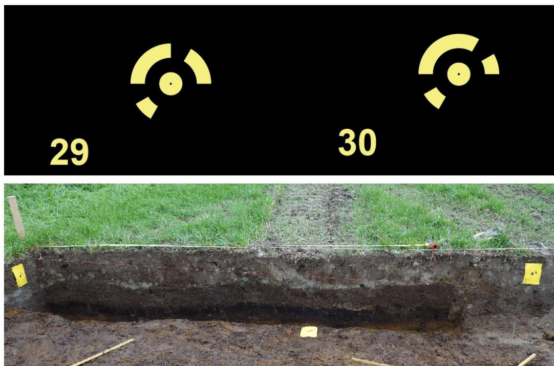
Figure 2. Photoscan provides coded markers which can be exported and printed. In the future, photogrammetric recording at BBC should be performed using coded markers. These can be automatically detected by PhotoScan when they appear in images. Using a colour combination that reduces the chance of overexposure is important when flash photography is performed.
