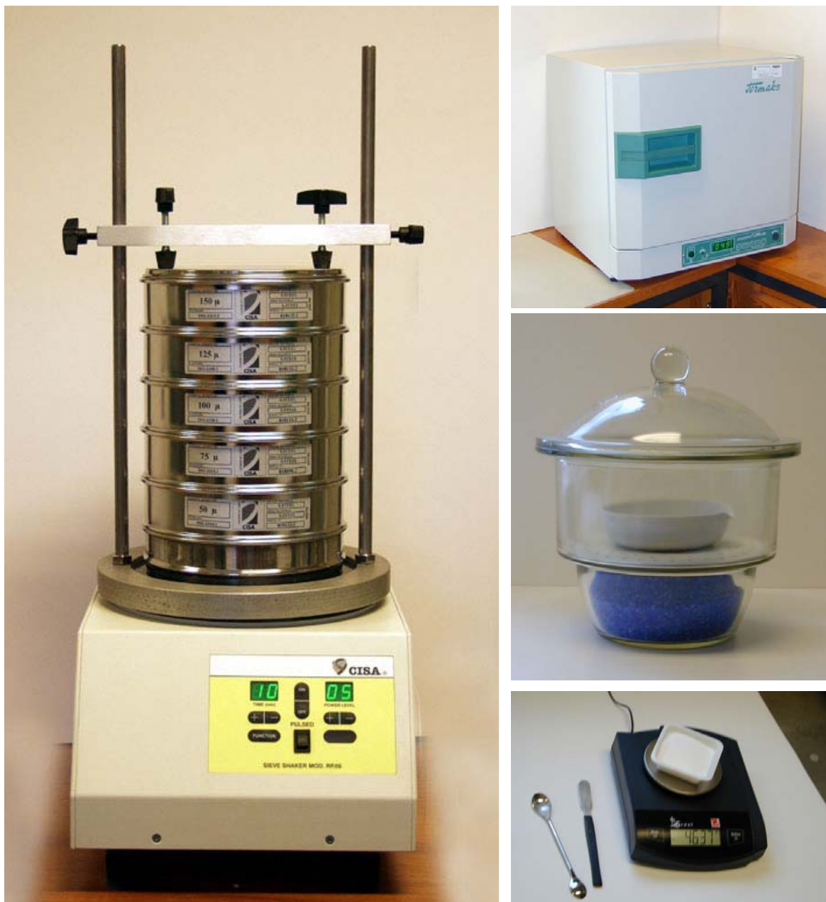
Figure B-15 The sieve shaker, with a stack of sieves (left); the drying oven (upper right); the desiccator (middle right); the electronic balance, with spoon and spatula (lower right).
