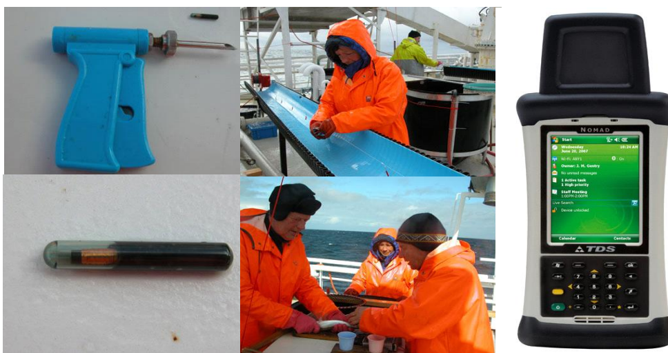
Figure 6: The tools used to insert RFID tag (top left), the glass encased RFID tag (bottom left), the slide used to release mackerel after tagging (top right) and the handling of the mackerel (bottom right) collectively show the process of tagging and releasing an individual. The data can be read and edited using the handheld PDA.
