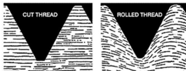
Figure 6: Cut thread vs rolled thread.
