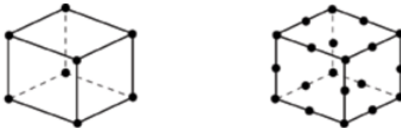
Figure 27: Linear C3D8 Element (left), Quadratic C3D20 Element (right)
