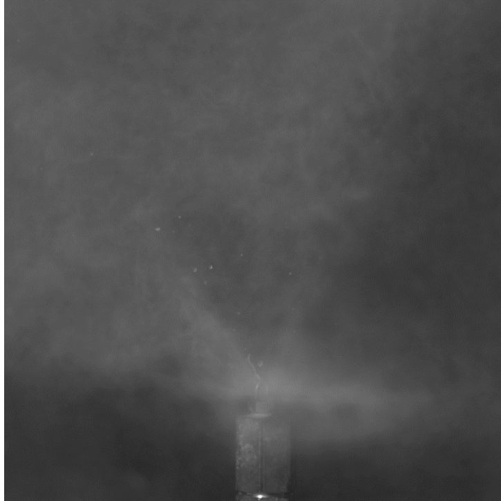
Figure B.1: Onset of water mist behaviour, 10 ms after injection with a flow rate of \approx 0.031 l/min.
