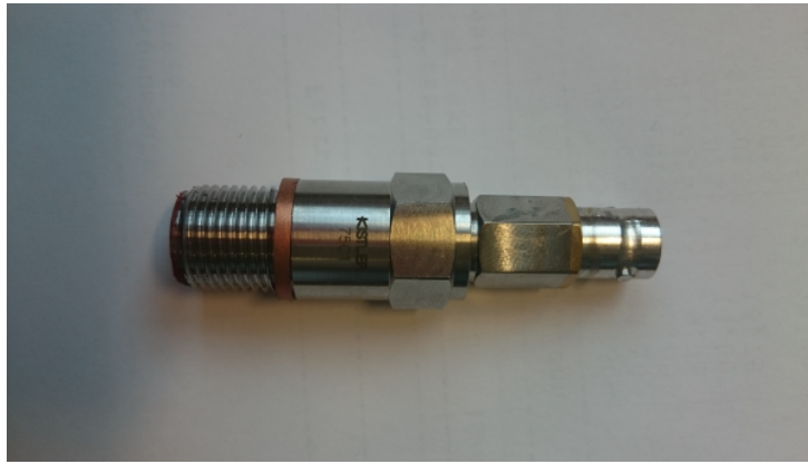
Figure 4.2: From left to right - Piezoelectric pressure sensor (Kistler 7031); Mounting adapter (Kistler 7501); BNC-mounting nipple (Kistler 7401).
