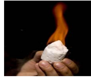
Figure 1.1 - Natural gas hydrates burning. [2]
