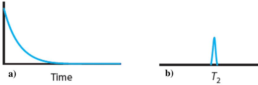
Figure 1.20 – a) The decay curve for T_2 relaxation time [26]. b) T_2 relaxation time distribution from analysis with the inverse Laplace transformation [26].
