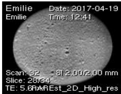
Figure 3.7 - Oil-wet sand containing heptane and water. The RAREst image is from the coronal orientation and displays slice 28 of 32.
