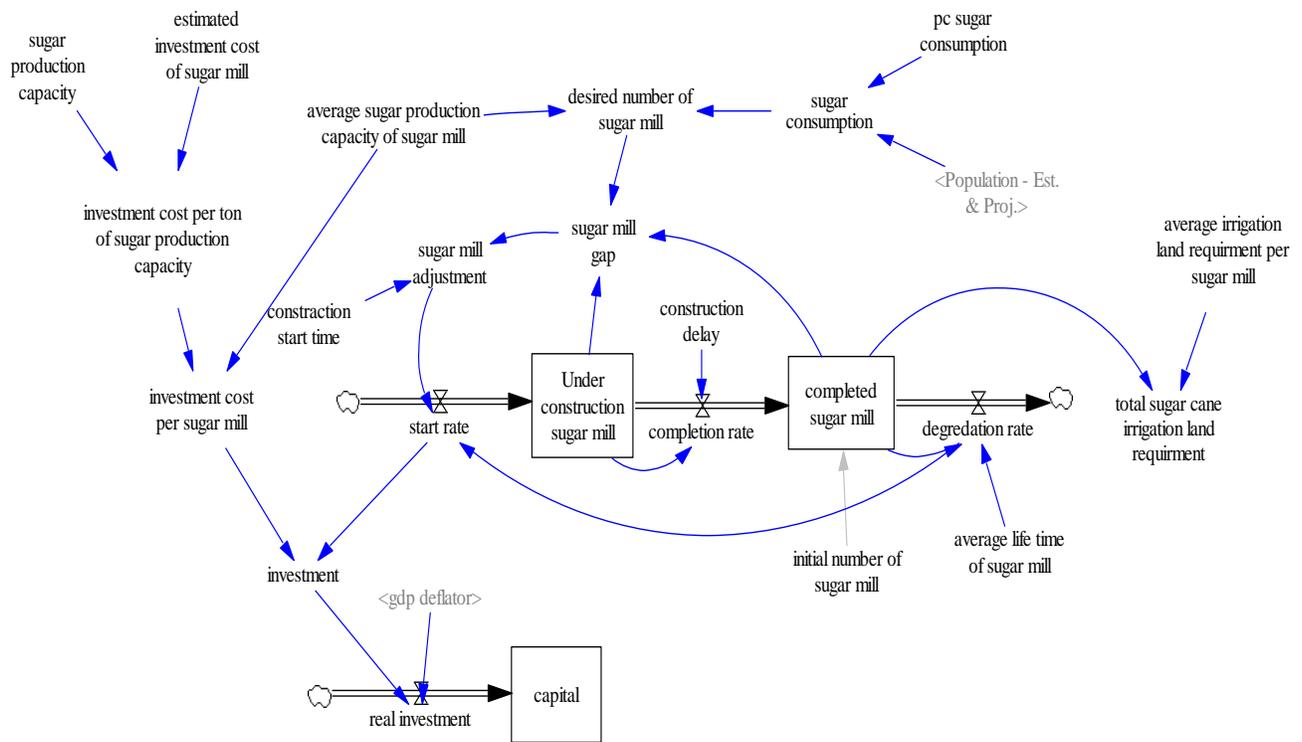
**Figure 16: Stock and flow structure showing construction of sugar factories**
