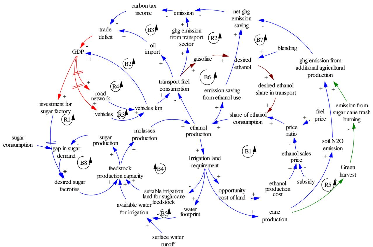
Figure 44: Main causal loop structure of the explanatory model (in blue and red) and the green harvest scenario (in green)
