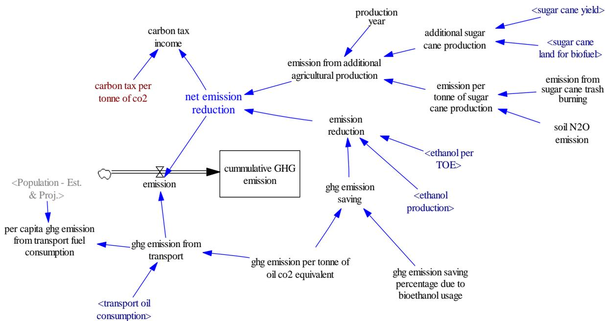
**Figure 20: Model structure showing transport sector GHG emission and GHG emission saving due to ethanol blending**
