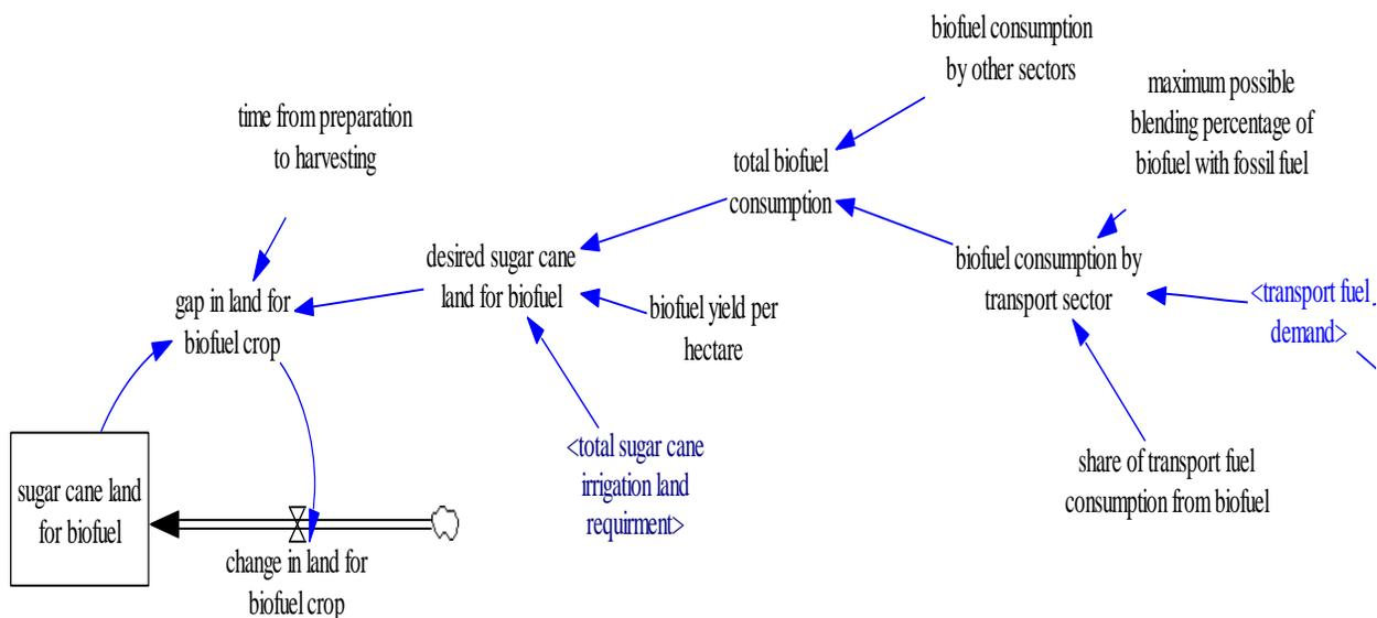
**Figure 10: Stock and flow structure of land for feedstock production**
