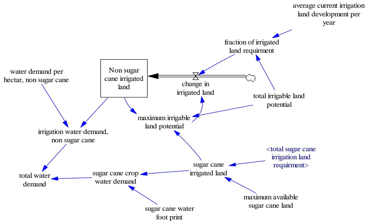
**Figure 18: Model structure showing land and water footprints for irrigation**
