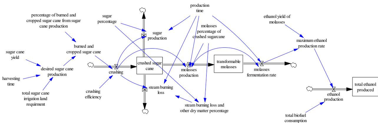
**Figure 14: Stock and flow structure of ethanol production process**
