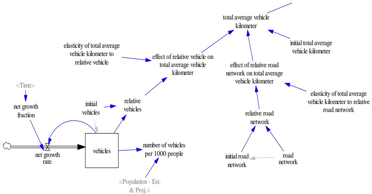
**Figure 5: Stock and flow structure of transport sector oil consumption**
